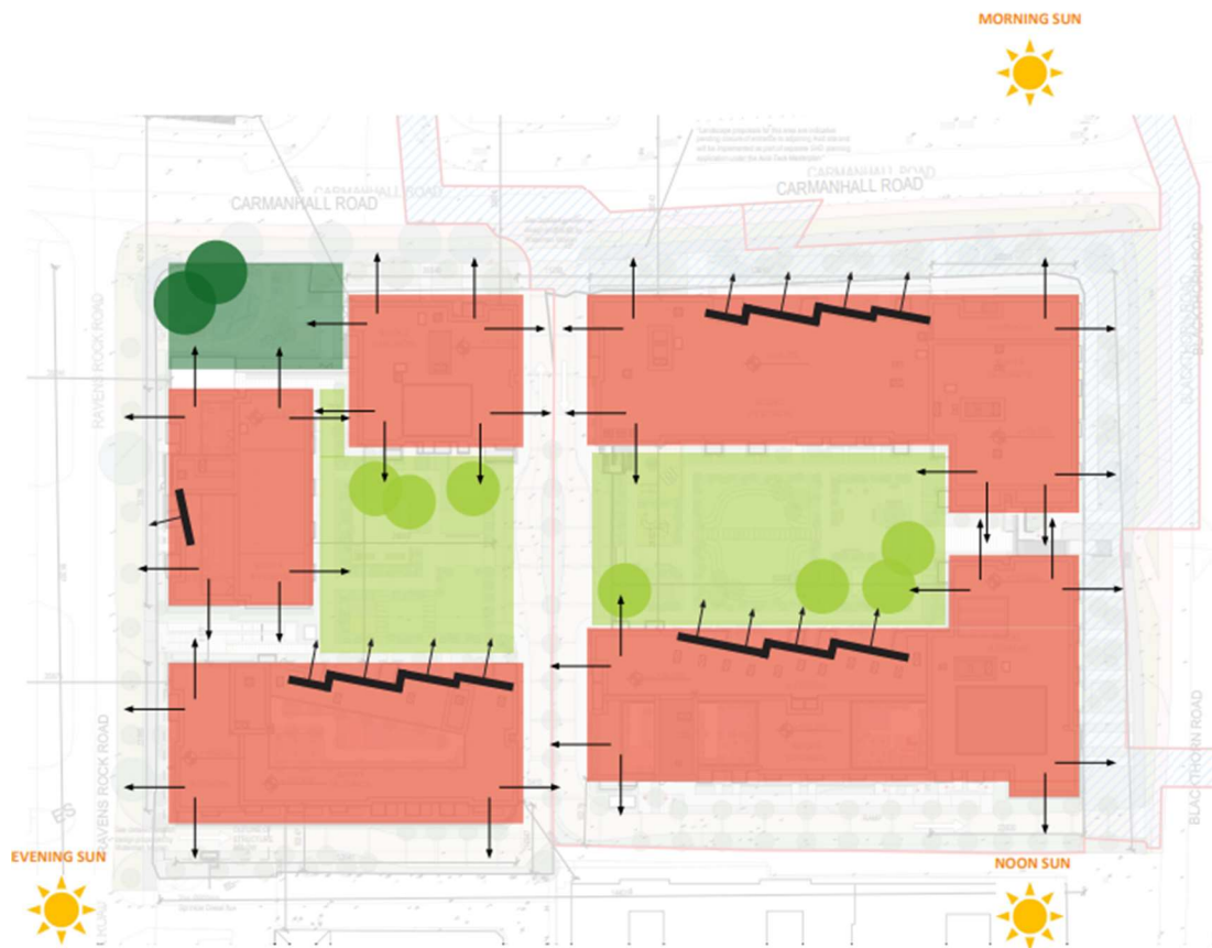
Figure 7: Solar Path Diagram (source: MDO – Architect Design Statement)
